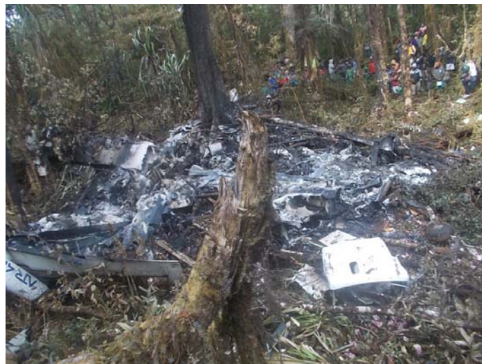
Figure 7: The wreckage of the fuselage damaged by post-impact fire
