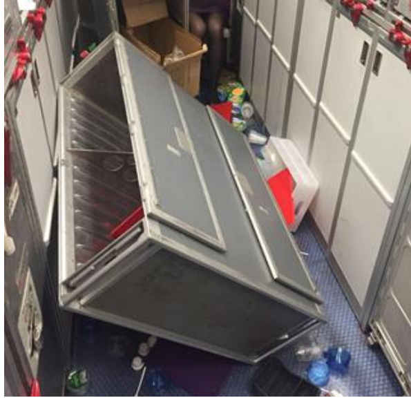
Figure 10: The aft galley condition after encounter turbulence
