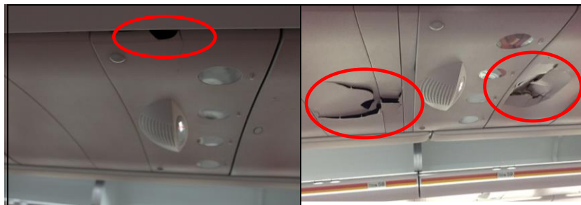
Figure 11: Damage on passenger service units
