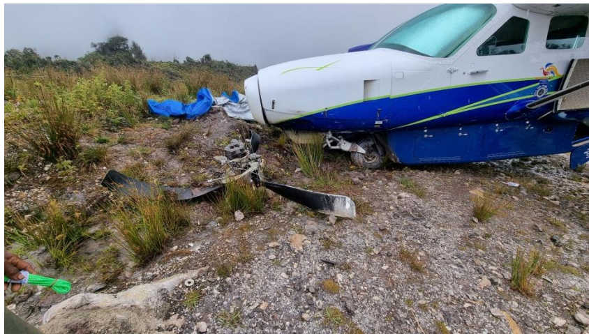
Figure 8: The detached propeller was adjacent to the aircraft
