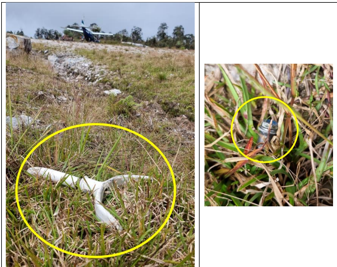
Figure 6: The fragment of the nose landing gear spring (drag link spring) and the broken bolt used for the nose gear spring attachment
