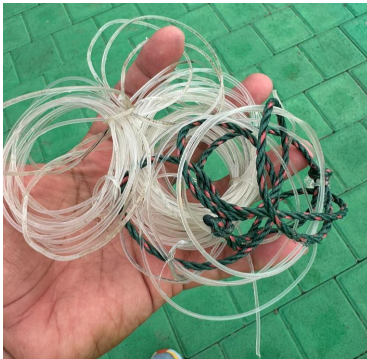
Figure 10: The kite string and plastic rope that were removed from main rotor and tail rotor masts
