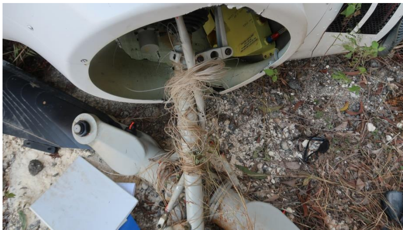
Figure 6: The evidence of kite string on the main rotor and tail rotor mast.
