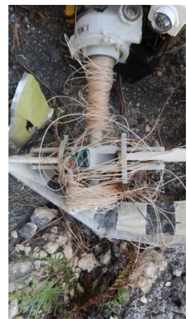
Figure 6: The evidence of kite string on the main rotor and tail rotor mast.
