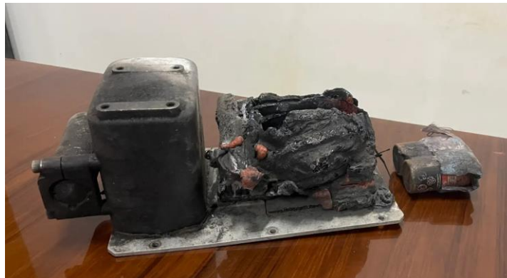
Figure 3: The CVFDR recovered from the accident site
